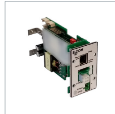
S-COM REMOTE CONTROL BOARD
