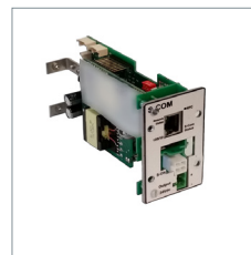
S-COM REMOTE CONTROL BOARD
